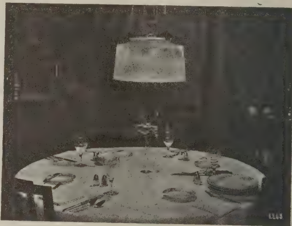
Fig. 4. A type of modern dome which is not too large and which may be hung sufficiently high
